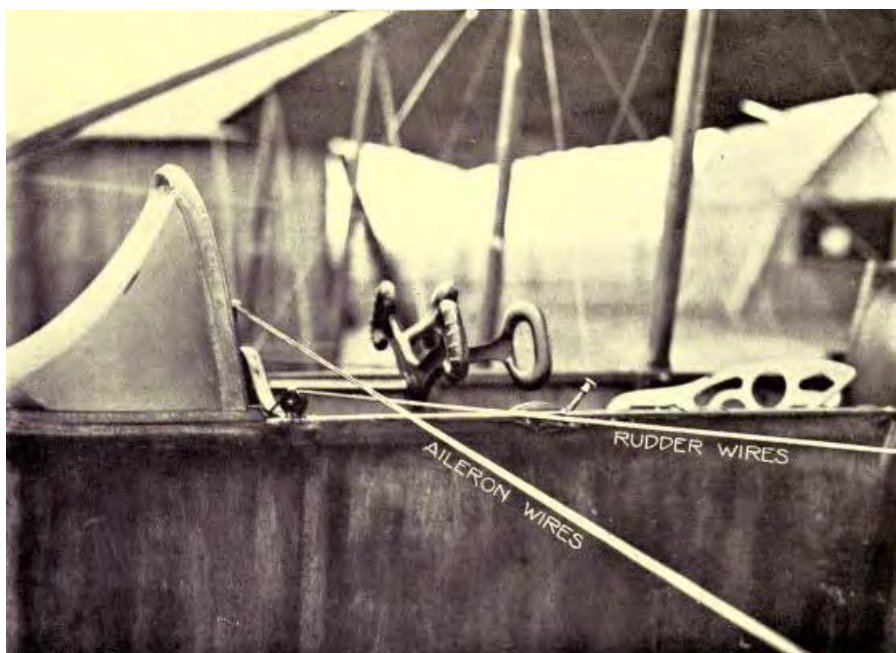
The double-handled control bar used on a school machine (Photo by Rameau, Étampes)
