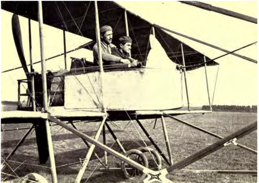
Pupil seated behind pilot, and holding the secondary pair of handles (Photo E. Rameau, Étampes)
